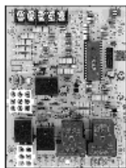
INTEGRATED FURNACE CONTROL
