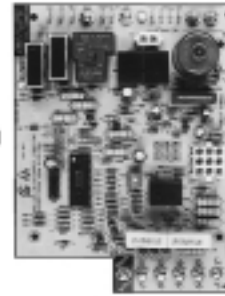
INTEGRATED FURNACE CONTROL
